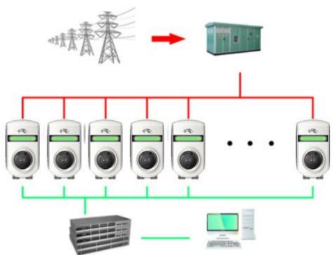
Ethernet version is connected to the switch by standard crystal head (RJ-45), and the main computer is directly connected to the wiring mode.
