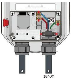
The device must be grounded. The fire wire (L) neutral wire (N) must be tested with the test pencil. The electric pen test is lit by the fire wire (L), and then the L wire and the N wire are respectively connected to the corresponding terminals!
